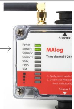
7. **The logger will take one reading when powered on and report it straightaway. After that, it will operate a default 15-minute read with a two hour upload or according to the interval set. So, after the first power on read, the first data will be available to download two hours later and every two hours thereafter. They can be verified using the web portal, SMS or WAP.**
