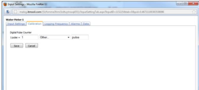
The Digital Pulse Counter calibration allows you to assign a real world value to every pulse of the sensor. The textboxes provided have the following layout: "1 pulse = [quantity][units of the quantity][if units of quantity is 'other' – enter the custom unit here]".
