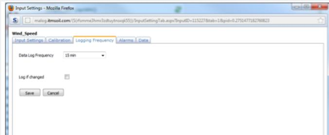
The Logging Frequency tab allows you to change the rate at which the input is read.
