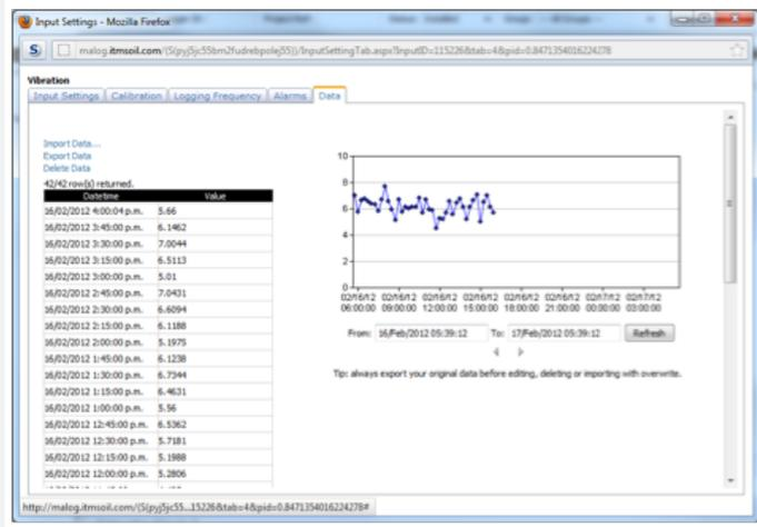
The Data tab allows you to quickly view data from the input. You will see both a tabular and a graphical view of the selected range of data.
