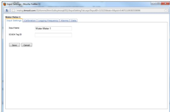
The Input Settings page has five tabs: Input Settings, Calibration, Logging Frequency, Alarms, and Data. There is a tab for every configurable column in the Native Inputs panel of the Sensor Configuration Page.
