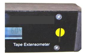
During this operation, the Tape Extensometer should be physically moved either side of the median position to ensure that any hysteresis within the instrument is eliminated. The correct tension is obtained when there are no visible yellow on either side of the black cursor line, and when any slight displacement to the extensometer reads as a positive displacement of the cursor line.
