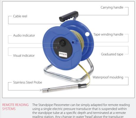
can be detected and related to the pressure at the piezometer tip.
